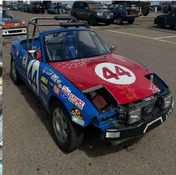
Figure 7: Intake system in context
