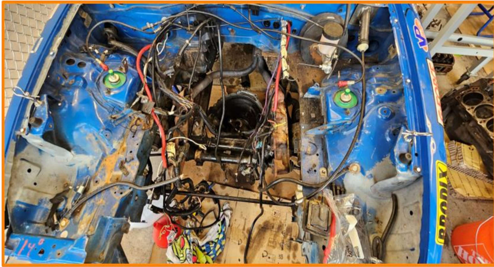
Figure 30: An image of the wiring harness in the empty hood.
