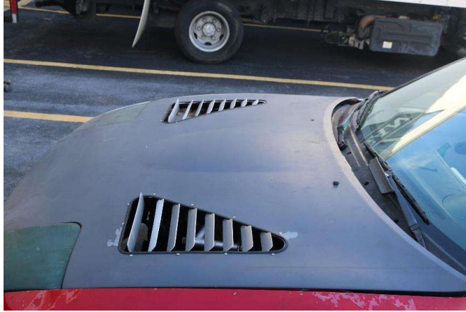
Figure 11: Potential hood vent locations [11]
