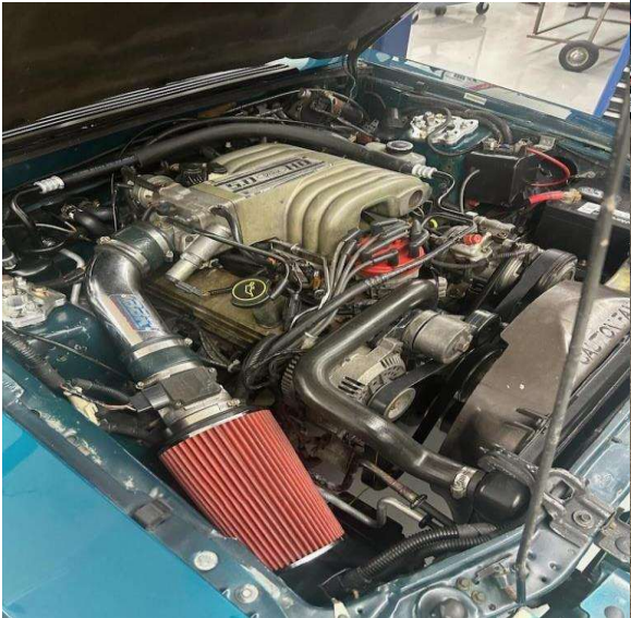
Figure 6: Example of a ram air intake
