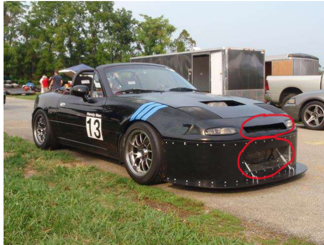
Figure 12: Potential Ducting Locations [12]
