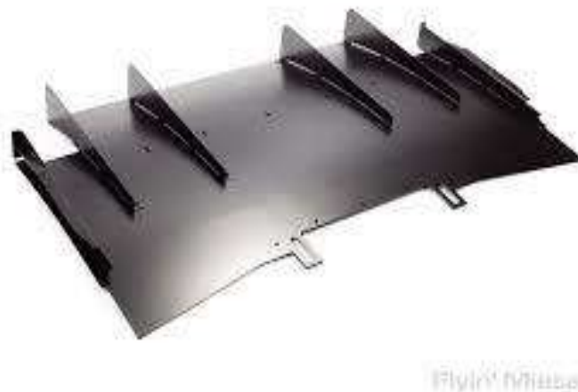
Figure 38: Miata Rear Diffuser Kit [47]
