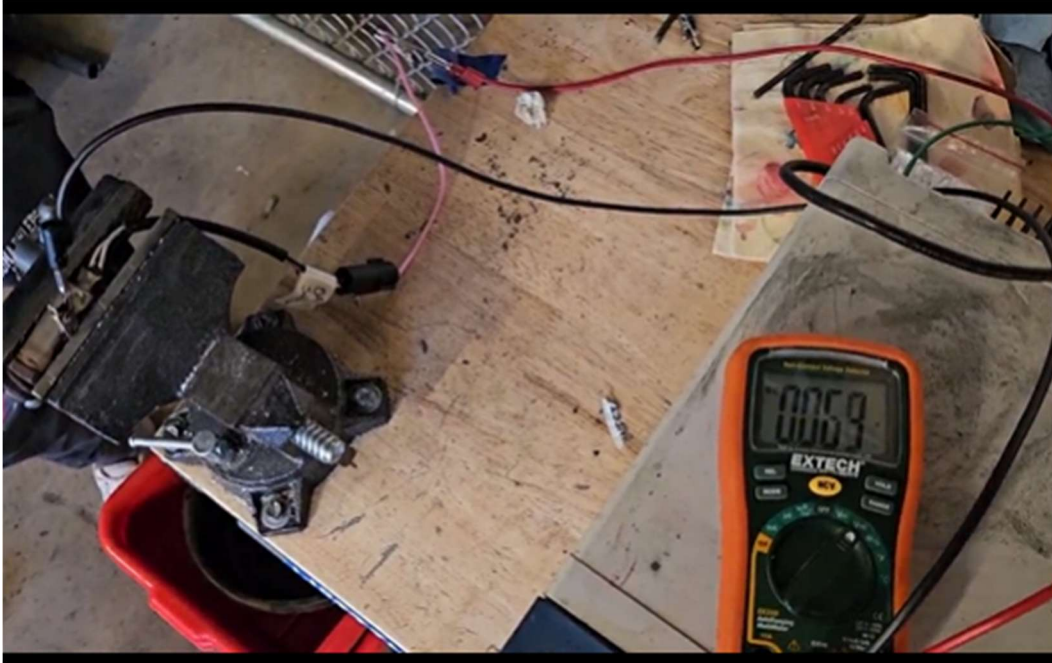
Figure B2-7: Voltage Reading After 5 Seconds of Heating
