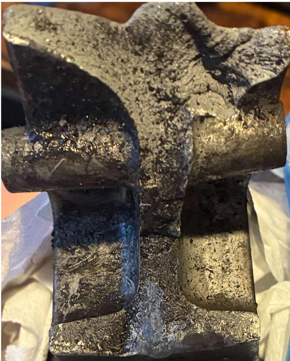
Figure 51: Strong-side failure face
