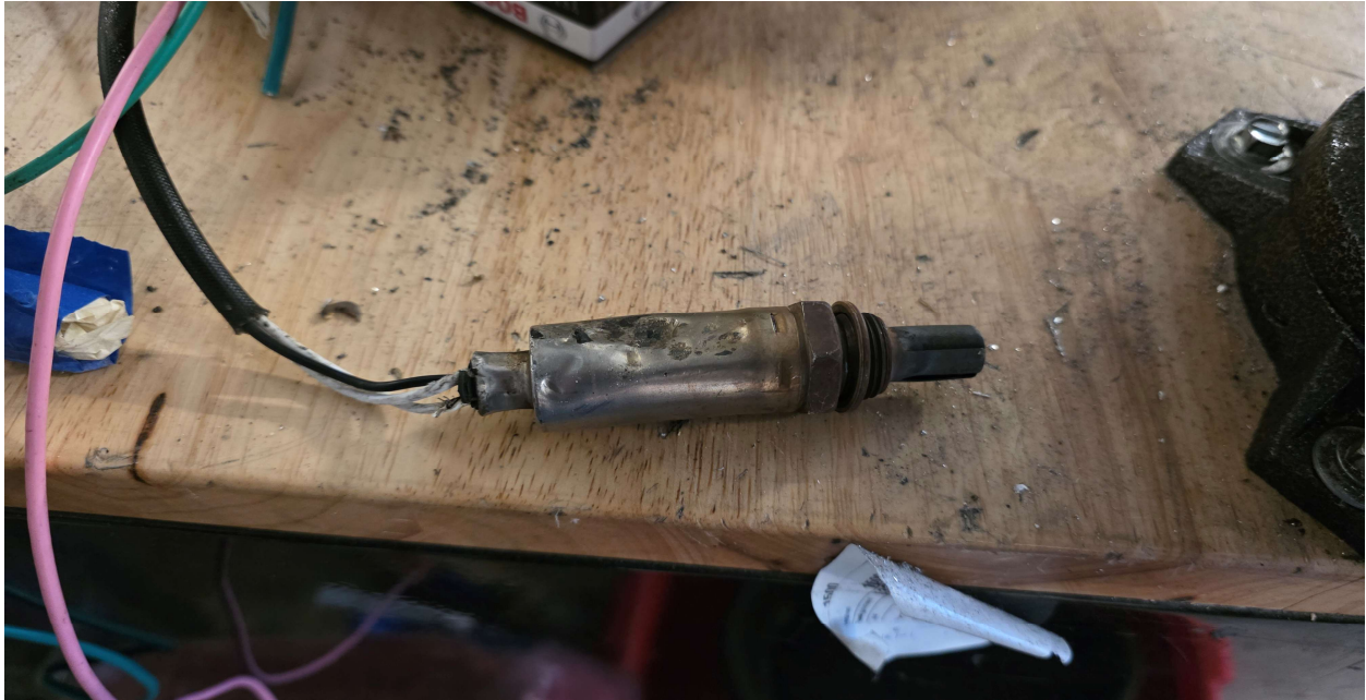
Figure B2-3: Physically Damaged O2 Sensor
