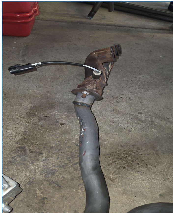
Figure B2-4: O2 Sensor Placement in Exhaust Manifold
